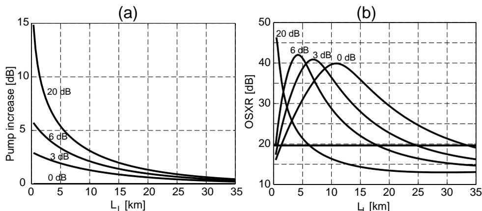
Fig. 2. (a) Pump increase  $P_{0I}/P_0$ , and (b)  $OSXR_I$  vs. isolator location  $L_I$ .
