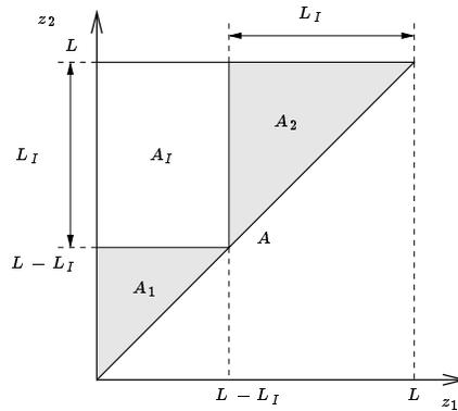
Fig. 1. Integration domain when an ideal isolator with bypass is placed  $L_I$  meters from the output.
