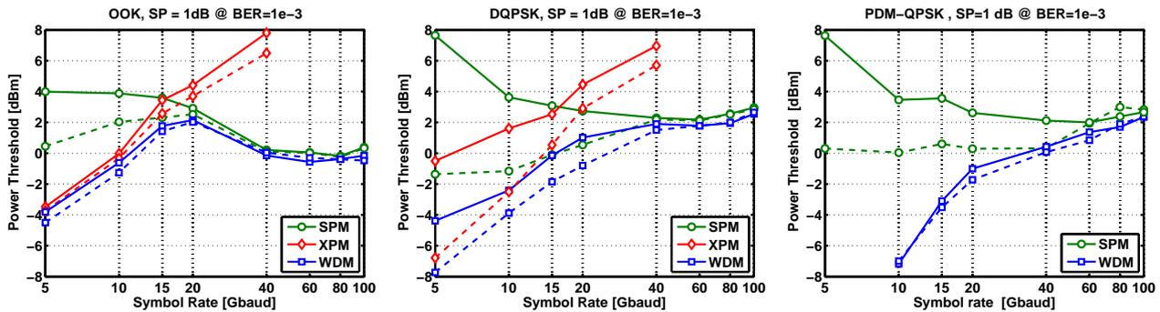
Fig. 2: Power threshold for SMF DM line for: (left) NRZ-OOK, (center) NRZ-DQPSK, (right) coherent PDM-NRZ-QPSK. Solid: no NSNI. Dashed: with NSNI. "SPM"= single-channel; "XPM"=no SPM, no FWM; "WDM"=all nonlinear effects.
