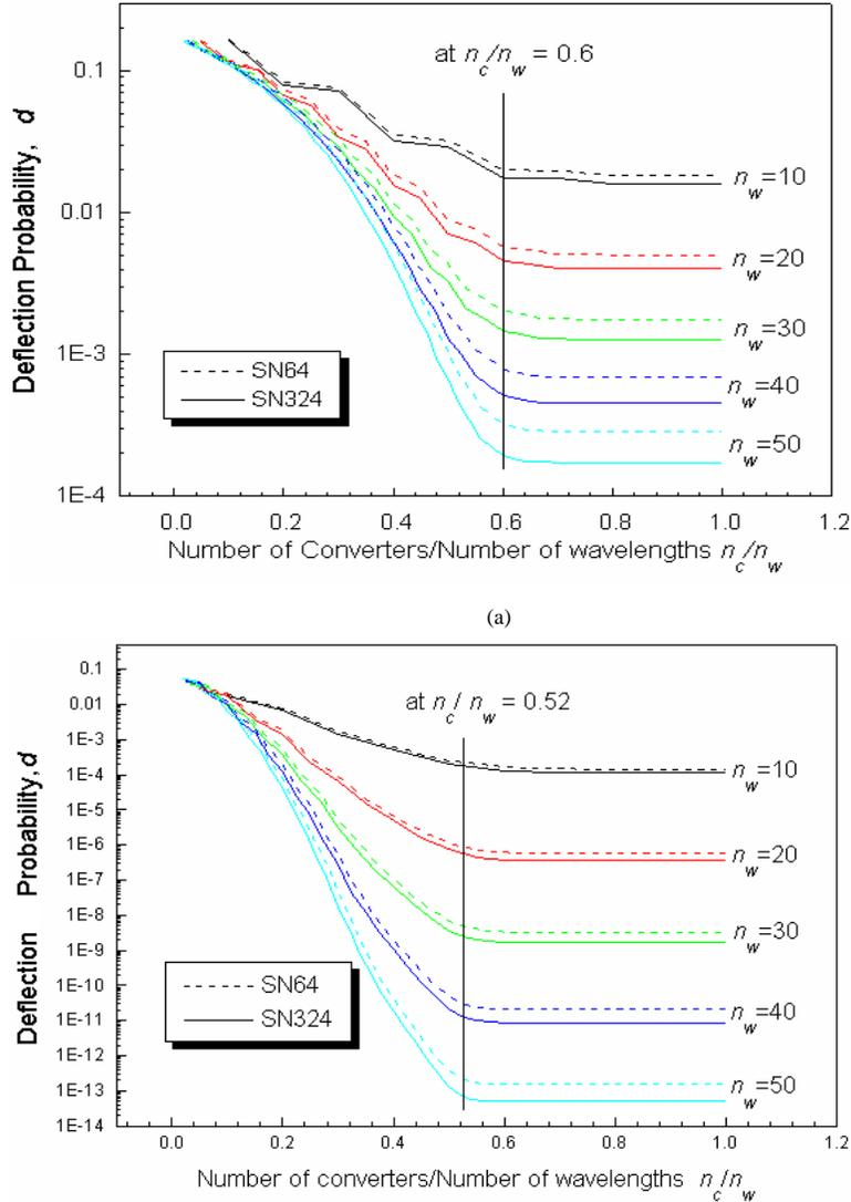
Fig. 5. (a) Deflection probability  $d$  versus number of converters/number of wavelengths ( $n_c/n_w$ ) when  $u = 1.0$ . (b) Deflection probability  $d$  versus Number of number of converters/number of wavelengths ( $n_c/n_w$ ) when  $u = 0.5$ .
