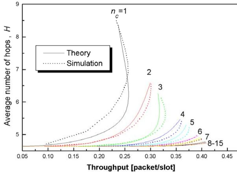
Fig. 2. Average number of hops  $H$  versus throughput per wavelength  $T$  for case  $n_w = 15$  wavelengths.
