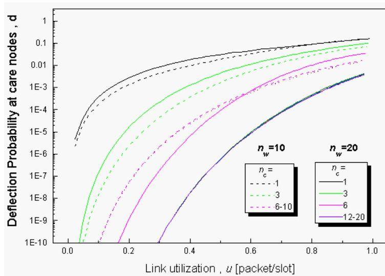
Fig. 4. Deflection probability at care nodes  $d$  versus link utilization  $u$  [packets/slot].
