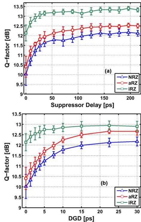
Fig. 2.  $Q$ -factor versus: (a) suppressor delay  $D$  at zero DGD, and (b) average DGD without suppressor, for a 19-channel PDM-QPSK  $20 \times 100$ -km SMF DM link with pulse formats NRZ, aRZ and iRZ (symbol time = 35.7 ps).
