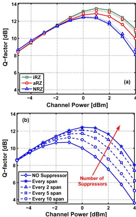
Fig. 4.  $Q$ -factor versus power for a 19-channel PDM-QPSK DM link with (a) XPM suppressor at all spans (ten-symbol delay) with average DGD = 0 ps (solid line) and 22.5 ps (dotted line). (b) NRZ-PDM-QPSK: DM link, DGD = 0 ps and XPM suppressor at all spans (stars), every ten spans (circles), every four spans (squares) and every other span (triangles).
