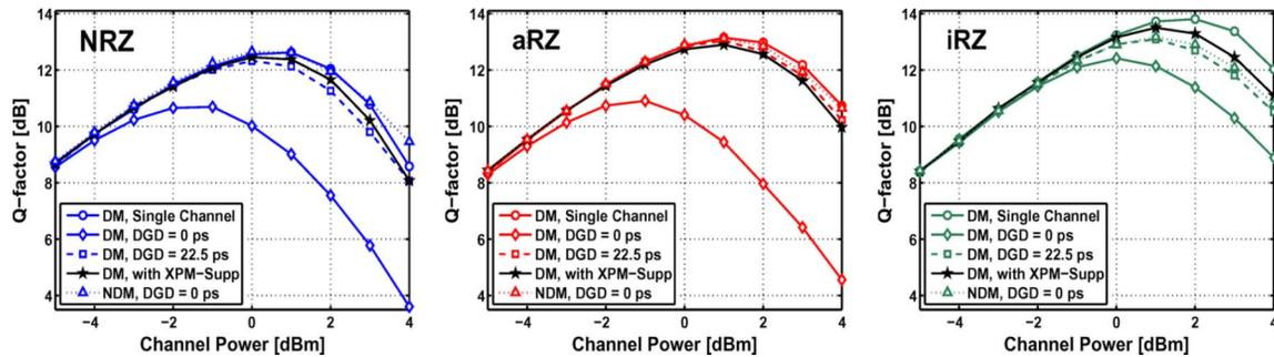
Fig. 3. Average  $Q$ -factor versus channel power for a 19-channel PDM-QPSK  $20 \times 100$  SMF link for different pulse formats and average DGD values. Black curves (stars) for XPM-suppressor calculated with  $D = 10$  symbols,  $DGD = 0$  ps.
