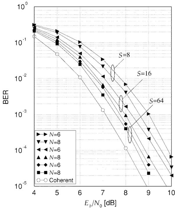
Fig. 2. BER of the proposed detection schemes for eight-state TC-16-QAM.
