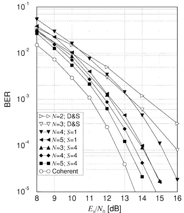
Fig. 1. BER of the proposed detection schemes for 16-DQAM with various degrees of complexity and comparison with receivers in [6] (D&S).
