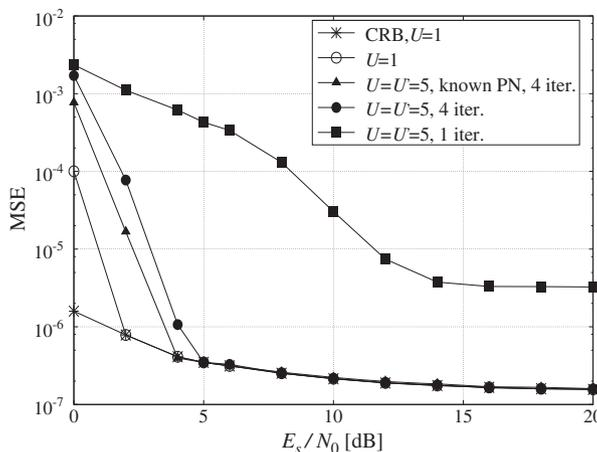
Figure 6. MSE of the multiuser frequency synchronization scheme in the presence of PN.
