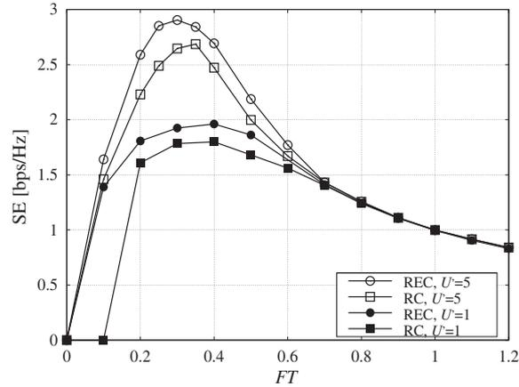
Figure 3. Spectral efficiency as a function of the normalized spacing for different values of  $U'$  at  $E_s/N_0 = 10$  dB.
