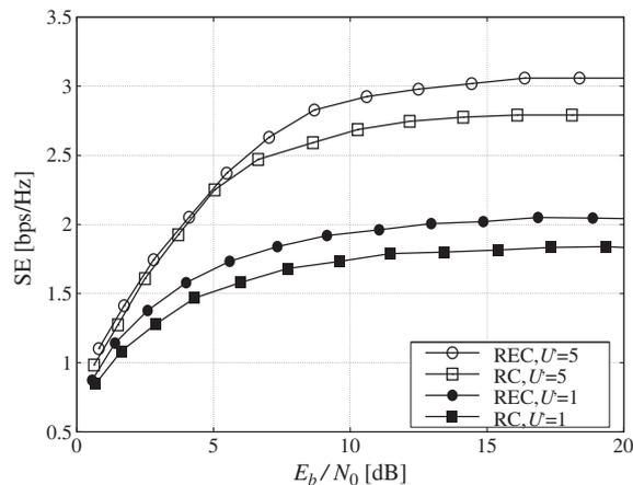
Figure 4. Spectral efficiency as a function of  $E_b/N_0$ , for channel spacings resulting from the optimization at  $E_s/N_0 = 10$  dB.
