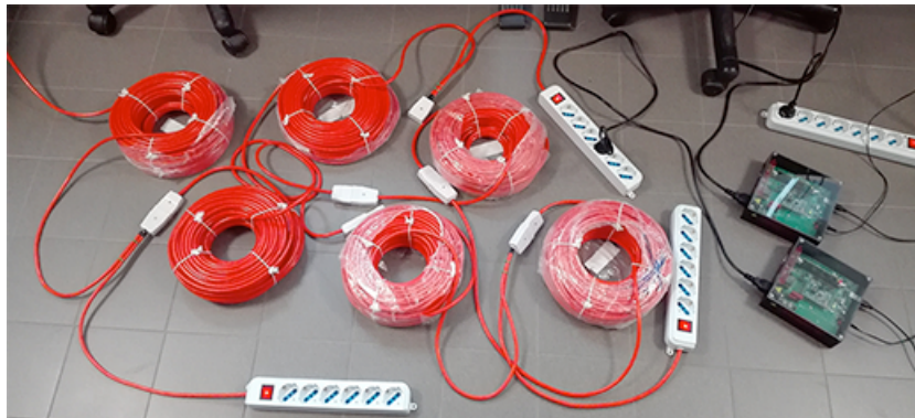
Fig. 13.6. Real deployment of an electrical line composed by different pieces of electrical cable.
