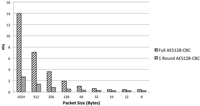
Figure 5.5: Decryption time as a function of the packet size.
