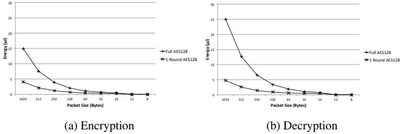
Figure 5.6: Comparison, in terms of consumed energy as a function of packet size, considering full and 1-round AES128-CBC.
