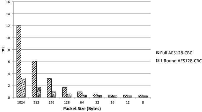
Figure 5.4: Encryption time as a function of the packet size.
