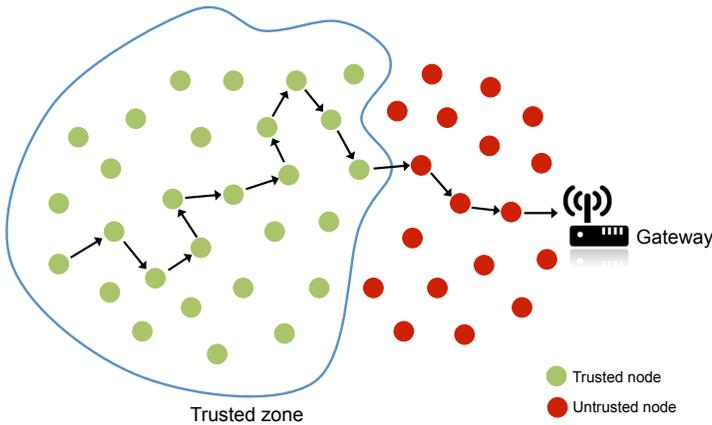
Figure 5.2: Multi-hop network: distributing block-ciphers computations among the trusted nodes.
