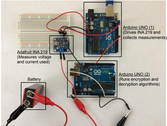
Figure 5.3: Arduino testbed used for the experiments.
