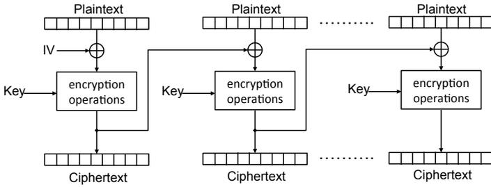
Figure 5.1: Example of block cipher iterative structure in Cipher Block Chaining (CBC) mode.
