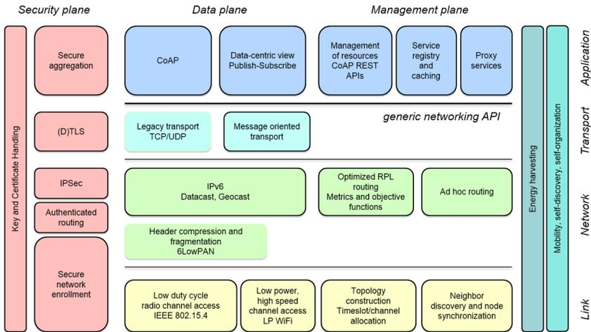
Figure 8.3 High level functional architecture of sensors
