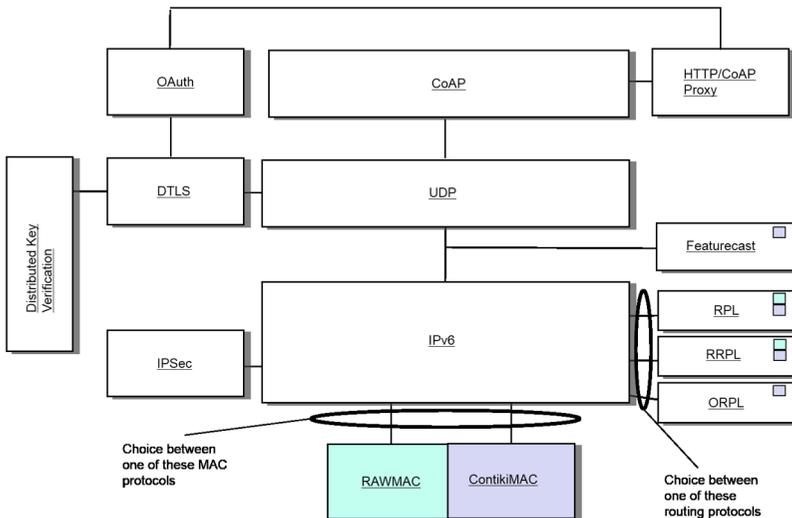
**Figure 8.7** Software architecture for Smart Parking
