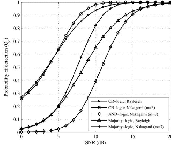
**Fig. 1.2** Probability of detection as a function of the average S-channel SNR ( $\bar{\gamma}_s$ ), considering various fusion rules (OR, AND, majority logic). Both Rayleigh and Nakagami- $m$  fading scenarios are considered. In all cases,  $N=3$  CR users,  $Q_f=0.1$ , and  $u=5$ .
