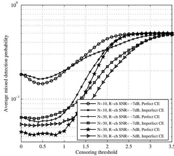
**Fig. 1.8** Average missed detection probability as a function of  $C_{th}$  for various values of  $N$  and  $\bar{\gamma}_R$  under perfect and imperfect channel estimation in Rayleigh fading channel ( $\bar{\gamma}_S = 20$  dB,  $P_f = 0.05$ , and  $u=5$ ).
