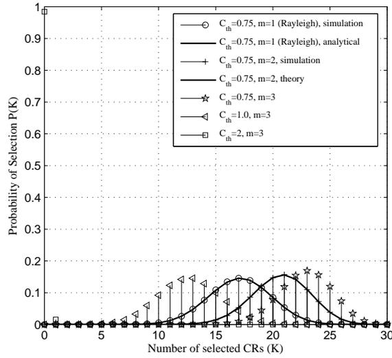
**Fig. 1.10** PMF of the number of censored CR users for different censoring thresholds ( $C_{th}$ ) under perfect channel estimation in Nakagami- $m$  faded channel.
