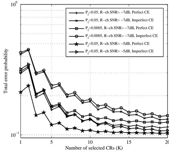
**Fig. 1.5** Total error probability versus the number of selected CR users ( $K$ ) under perfect and imperfect channel estimation for various values of ( $\bar{\gamma}_R$ ) and  $P_f$  in Rayleigh fading ( $\bar{\gamma}_s=20$  dB,  $N=20$ , and  $u=5$ ).
