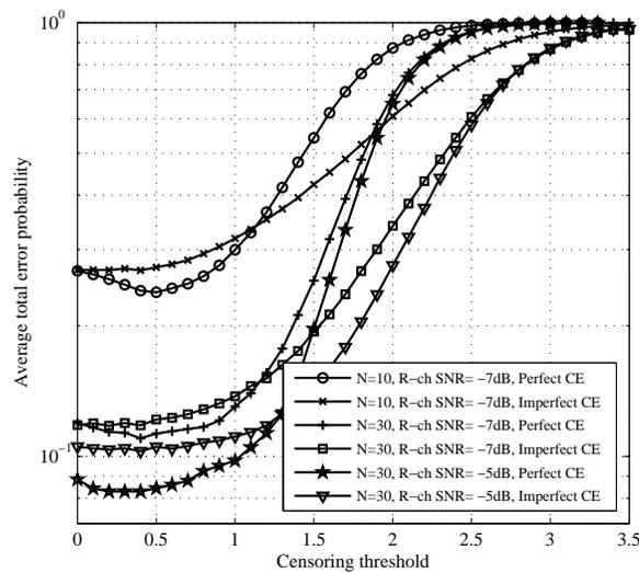
**Fig. 1.9** Average total error probability as a function of  $C_{th}$  for various values of  $N$  and  $\bar{\gamma}_R$  under perfect and imperfect channel estimation in Rayleigh fading channel ( $\bar{\gamma}_i=20$  dB,  $P_f=0.05$ , and  $u=5$ ).
