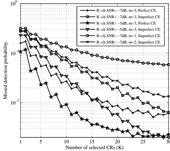
**Fig. 1.6** Performance of CSS with censoring of CR users under perfect and imperfect channel estimation for various values of average R-channel SNRs ( $\bar{\gamma}_R$ ) in Nakagami- $m$  faded environment, impact of fading parameter ( $m$ ) on imperfect channel estimation is also depicted ( $\bar{\gamma}_s=20$  dB,  $N=30$ ,  $P_f=0.05$  and  $u=5$ ).
