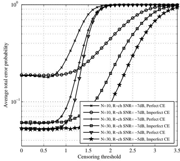
**Fig. 1.12** Average missed detection probability as a function of  $C_{th}$  for various values of  $N$ , and  $\bar{\gamma}_R$  under perfect and imperfect channel estimation in case of Nakagami- $m$  fading ( $\bar{\gamma}_S=20$  dB,  $m=3$ ,  $P_f=0.05$ , and  $u=5$ ).
