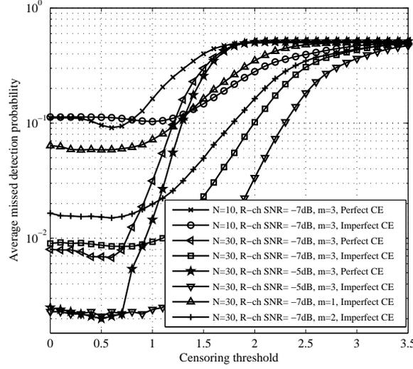
**Fig. 1.11** Average missed detection probability as a function of  $C_{th}$  for various values of  $N$ ,  $m$  and  $\bar{\gamma}_R$  under perfect and imperfect channel estimation in case of Nakagami- $m$  fading ( $\bar{\gamma}_S=20$  dB,  $P_f=0.05$ , and  $u=5$ ).
