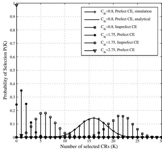
**Fig. 1.7** PMF of the number of censored CR users for different censoring thresholds ( $C_{th}$ ) under both perfect and imperfect channel estimation in Rayleigh faded channel.
