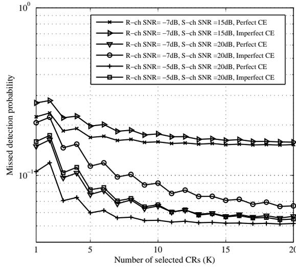
**Fig. 1.4** Performance of CSS network with censoring of CR users under perfect and imperfect channel estimation for various values of average R-channel SNR ( $\bar{\gamma}_R$ ) and average S-channel SNR ( $\bar{\gamma}_S$ ) in Rayleigh fading (CE stands for channel estimation,  $N=20$ ,  $P_f=0.05$  and  $u=5$ ).
