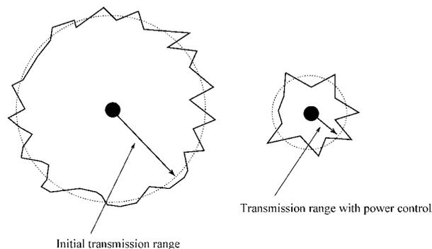
**Fig. 3** Impact of shadowing on the transmission area of a node: before power control (left) and after transmit power reduction (right)
