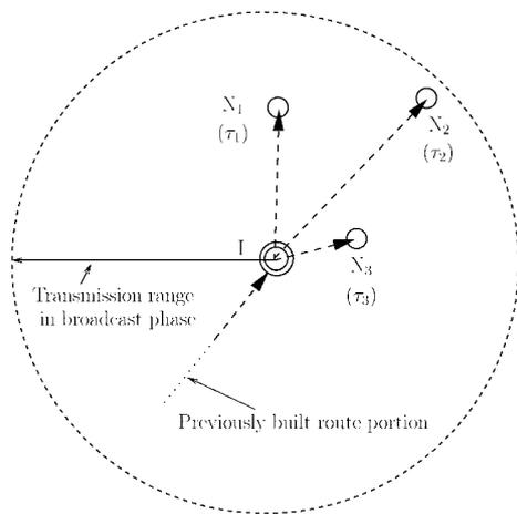
**Fig. 2** Intermediate forwarding during the broadcast phase: the RREQ packet sent from node I is received by nodes  $N_1$ ,  $N_2$  and  $N_3$ , which wait  $\tau_1$ ,  $\tau_2$  and  $\tau_3$  to retransmit. If the MAODV protocol is used, it holds that  $\tau_3 < \tau_1 < \tau_2$
