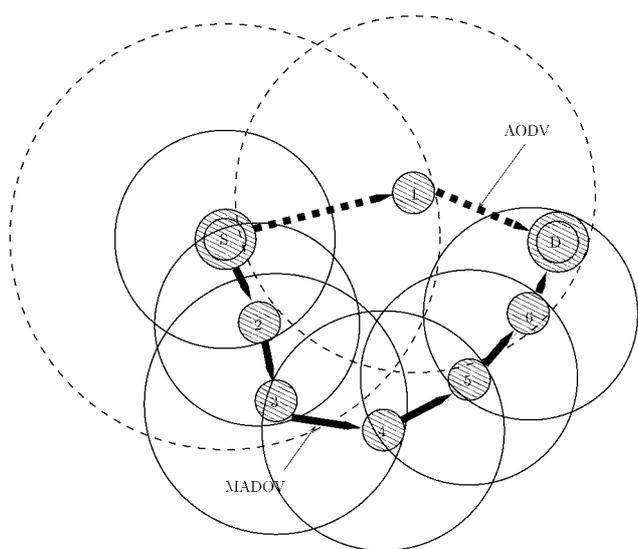
**Fig. 1** Routing strategies: MAODV (solid circles, centred at nodes, with radiuses equal to the corresponding nodes' transmission ranges) against AODV (dashed circles, centred at nodes, with radiuses equal to the corresponding nodes' transmission ranges)
