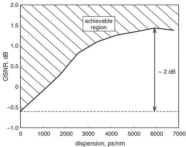
**Fig. 3** OSNR against dispersion at IR equal to 239/255
