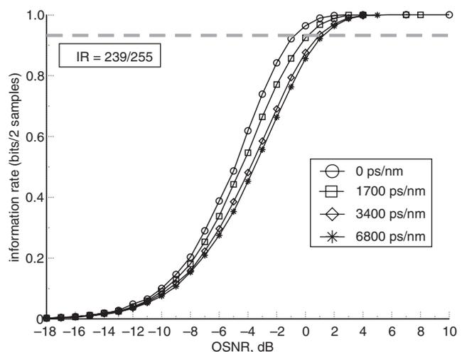
**Fig. 2** IR against OSNR at dispersion values 6800, 3400, 1700, 0 ps/nm
