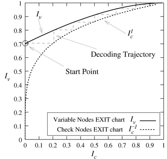
Fig. 2. EXIT chart for a regular (3,6) LDPC code transmitted over an AWGN channel with SNR equal to 1.8 dB. The dashed line represents the evolution trajectory of the MI.
