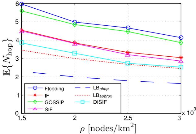
Fig. 14.  $\mathbb{E}\{N_{\text{hop}}\}$  as a function of  $\rho$ . The performances of the considered broadcasting protocols are directly compared with the bounds  $LB_{\text{nhop}}$  (Eq. (6)) and  $LB_{\text{approx}}$  (Eq. (11)).
