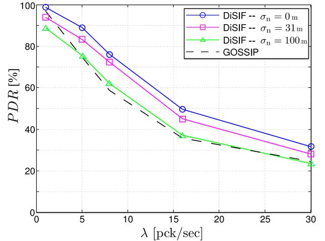
Fig. 15. DiSIF performance, considering the GPS positioning error, in term of  $PDR$  as function of  $\lambda$ . Three different values of  $\sigma_n$  are considered: 0, 31, and 100 m. For comparison purposes the performance of GOSSIP is also shown. The main network parameters are set as in Fig. 10.
