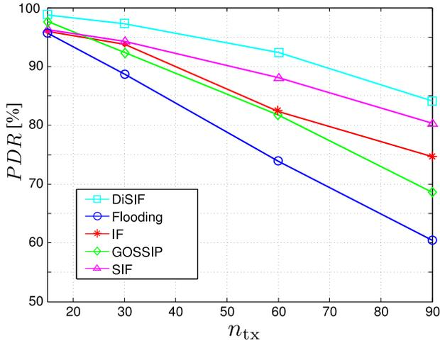
Fig. 11. *PDR* as a function of  $n_{tx}$ . Network parameters are set as follows:  $p_s = 128$  byte/pkt,  $\rho = 2,000$  nodes/km<sup>2</sup>,  $n = 150$  nodes,  $\lambda = 0.5$  pkt/s,  $s_p = 1.5$  m/s, and  $c = 1$ . Various broadcasting protocols are directly compared.
