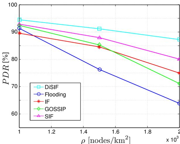
Fig. 12. *PDR* as a function of the nodes spatial density. Network parameters are set as follows:  $p_s = 128$  byte/pkt,  $n_{tx} = 80$  nodes,  $n = 200$  nodes,  $\lambda = 0.5$  pkt/s,  $s_p = 1.5$  m/s, and  $c = 1$ . Various broadcasting protocols are directly compared.
