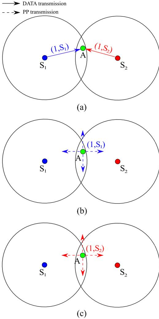
Fig. 5. Representative example of DiSIF propagation with two sources of information: (a) nodes  $S_1$  and  $S_2$  send DATA packet to  $A$ , (b) node  $A$  first rebroadcasts the PP with UID  $(1, S_1)$ , and (c) node  $A$  rebroadcasts the PP with UID  $(1, S_2)$ .
