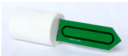
Fig. 9. nRF51822 SoC-based sensor node measuring soil temperature and soil moisture.
