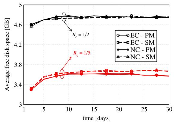
**Fig. 5.** Average free available disk space per StN, as a function of time, in a scenario with  $k = 50$ ,  $T_M = 30$  min,  $T_S = 3$  min, and  $q = 2^{16}$ . Different coding and maintenance strategies are considered.
