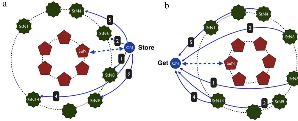
**Fig. 1.** The considered P2P overlay scheme with illustrative examples of (a) resource store and (b) resource retrieval process. In both cases, the resource consists of 5 fragments.
