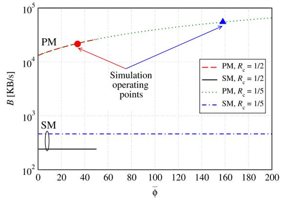
**Fig. 6.** Maintenance bandwidth, as a function of  $\bar{\phi}$ , in a scenario with  $k = 50$  with either PM with  $T_M = 30$  min or SM with  $T_S = 3$  min. Two values  $R_c$  for the coding rate are considered: 1/2 or 1/5. Other parameters are obtained through simulations.
