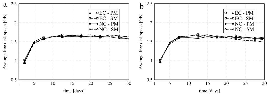
**Fig. 7.** Average free available disk space per StN, as a function of time, in a scenario with  $k = 50$ ,  $R_c = 1/2$ ,  $T_M = 30$  min,  $q = 2^{16}$ , and the non-uniform file size distribution. The performance is analyzed for both  $T_s = 3$  min (case (a)) and  $T_s = 36$  s (case (b)). Different coding and maintenance strategies are considered.
