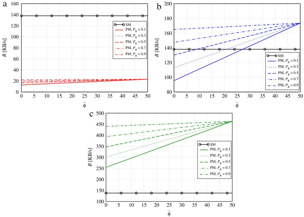
**Fig. 3.** Maintenance bandwidth (dimension: (kB/s)), as a function of  $\bar{\phi}$  (adimensional), in a scenario with  $k = 50$ ,  $R_c = 1/2$ ,  $\gamma = 10$ , with either PM (with  $T_M = 30$  min) or SM (with  $T_S = 3$  min). In case (a)  $N_{res} = 2$ , in case (b)  $N_{res} = 15$ , and in case (c)  $N_{res} = 40$ . Different values of  $P_R$  are considered in the PM scenarios.
