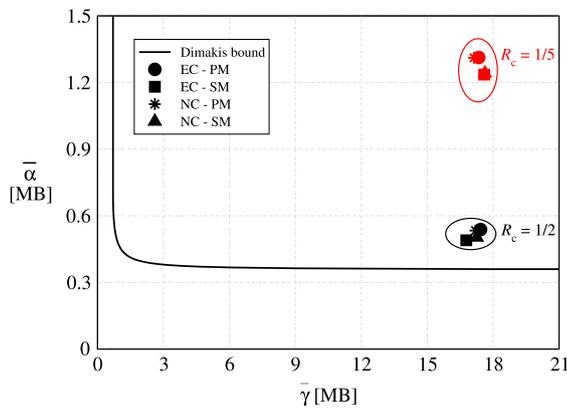
**Fig. 4.** Storage/repair tradeoff for resources of average size  $\bar{\gamma} = 18$  MB divided into 50 fragments coded with rate  $R_c = 1/2$  or  $R_c = 1/5$ . The operating points of different strategies are shown.
