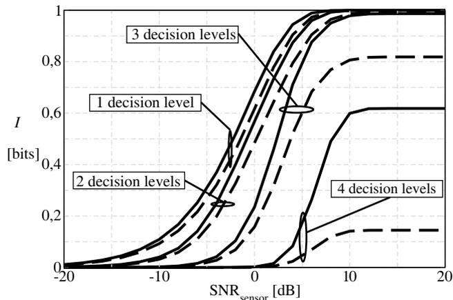
Fig. 3. Mutual information, as a function of the sensor SNR, in a sensor network with uniform clustering and noisy communication links with two possible values of the cross-over probability: (i)  $p = 0.01$  (solid lines) and (ii)  $p = 0.05$  (dashed lines).
