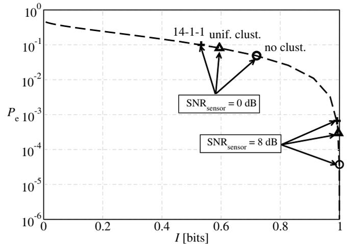
Fig. 2. Probability of decision error, as a function of the mutual information. The operational points for various clustering configurations and two sensor SNRs are shown.
