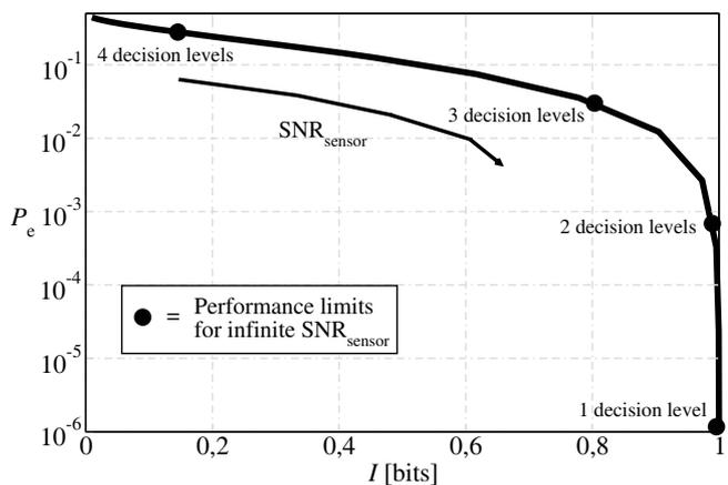
Fig. 4. Probability of decision error, as a function of the mutual information, in a scenario with uniform clustering and noisy communication links ( $p = 0.05$ ). The limiting ( $\text{SNR}_{\text{sensor}} \rightarrow \infty$ ) operational point with various number of decision levels are shown.
