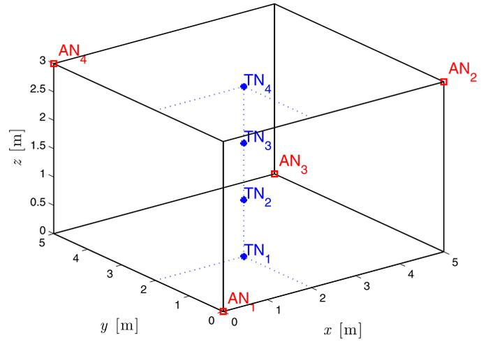
**Fig. 3.** Third experimental configuration: the positions of the ANs (red squares) and the various positions of the TN (blue dots) are shown. (For interpretation of the references to color in this figure legend, the reader is referred to the web version of this article.)
