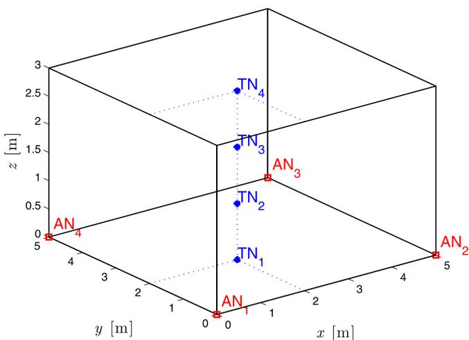
**Fig. 1.** First experimental configuration: the positions of the ANs (red squares) and the various positions of the TN (blue dots) are shown. (For interpretation of the references to color in this figure legend, the reader is referred to the web version of this article.)
