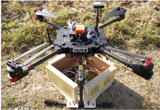
FIGURE 12. Flying UAV platform used for the flight tests and composed by the drone and the SSAS.
