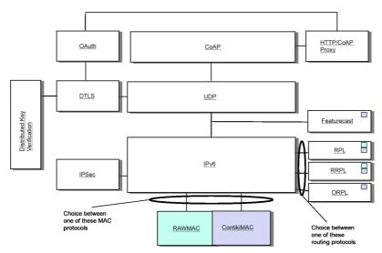
Figure 8.7 Software architecture for Smart Parking
