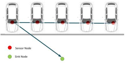
Figure 8.10 Configuration of the network topology
