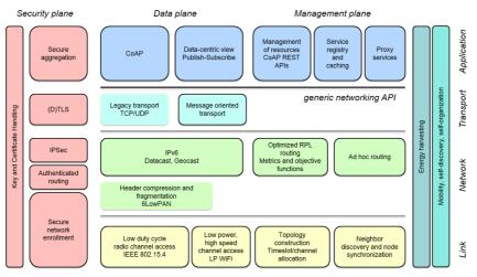
Figure 8.3 High level functional architecture of sensors
