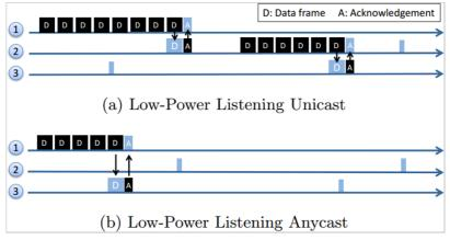
**Figure 8.5** Traditionally, routing uses unicast over stable links aiming at stability. Low-power listening introduces a significant delay at every hop. ORPL uses anycast and transmits to the first awoken forwarder that receives the packet regardless of link quality estimates
