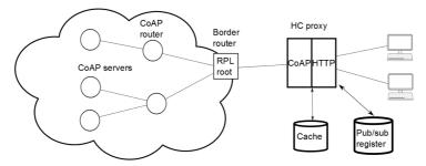
Figure 8.6 Scheme of the implemented HTTP/CoAP caching system
