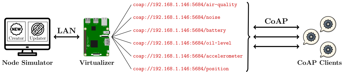
Fig. 7: Setup for the experimental evaluation of the proposed virtualization architecture, with the Virtualizer hosted on a RPi3. The experimental performance evaluation has also been carried out hosting the Virtualizer on a laptop.
