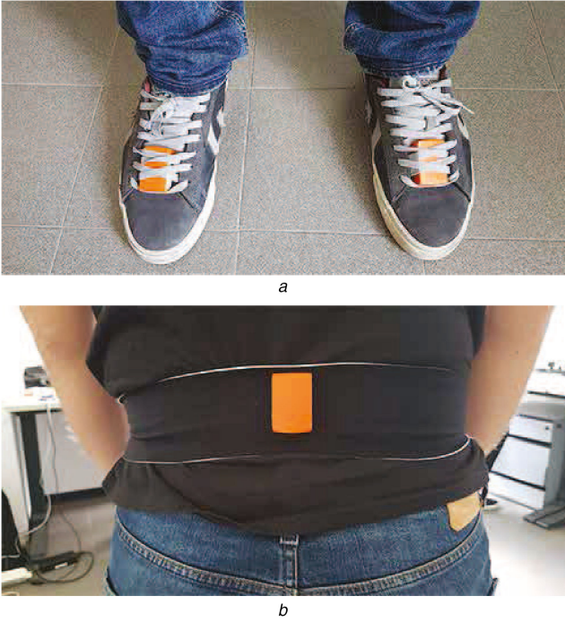
Fig. 1 Sensor positions: (a) the IMUs are mounted under the shoe-laces, one per foot; (b) the IMU is attached to a velcro band in the middle of the back, over the spine
