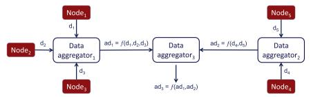
Fig. 3. In-network data aggregation.
