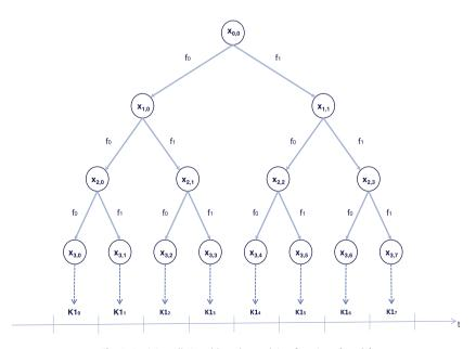
**Fig. 1.** Deriving all K1 subkeys by applying functions  $f_0$  and  $f_1$ .
