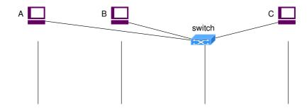
8) Considering the following network scheme, specify a possible message flow for a an ICMP spoofing attack of type "redirect", launched by a node C (attacker) trying to become Man In The Middle between nodes A (victim) and B. Particularly, consider the case in which A and B want to exchange the following 4 IP packets: pkt1:A\rightarrow B, pkt2:B\rightarrow A, pkt3:A\rightarrow B, pkt4:B\rightarrow A, and the attack starts when the first packet (pkt1) is sent.
