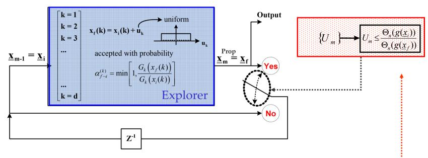
The d component-wise reject/accept Metropolis tests will thus produce correlated proposals  $\underline{x}_f$  with the desired distribution  $f_X(\underline{x})$ , so that the outer reject/accept mechanism has now a reasonable acceptance probability
