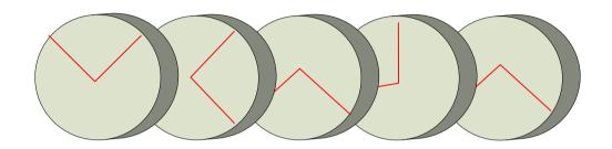
PMD fiber emulated with 25 PMF waveplates, each with a local DGD of 1 ps and uniformly distribted PSP over Poincarè sphere.
