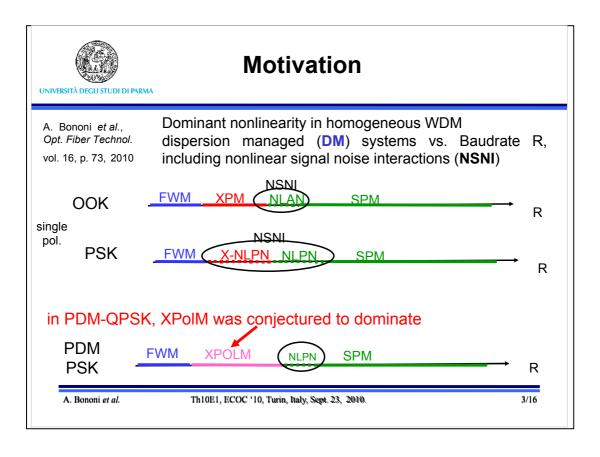
We presented last year at ECOC, and later in this OFT paper, a simulation study of the dominant nonlinearity in WDM homogeneous terrestrial DM systems as the signal baud rate was increased,
