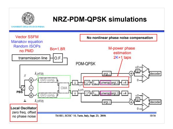
The vector SSFM simulation used the Manakov equation with random ISOPs and no PMD in the line.
