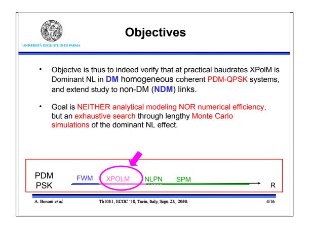
Hence the objective of this work is to indeed verify that XPoIM is the dominant nonlinearity in DM homogeneous
