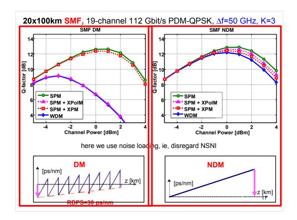
We now show the Q factor vs transmitted power, the so called bell-curves, for a 2000 km SMF line, with 19 PDM-QPSK channels at 28 Gbaud and 50 GHz channel spacing.
