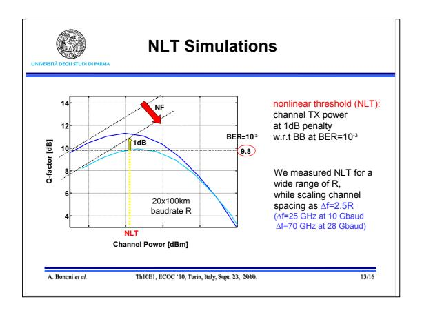
Next we show curves of nonlinear threshold NLT versus baudrate for the same 2000 km SMF line as before.
