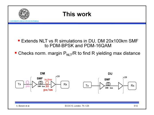
So in this work we extend the NLT vs R OFC'11 simulations to 2 more modulation formats, namely, BPSK and 16QAM, and we check the NLT/R curves to find the optimal R that yields the max distance.
