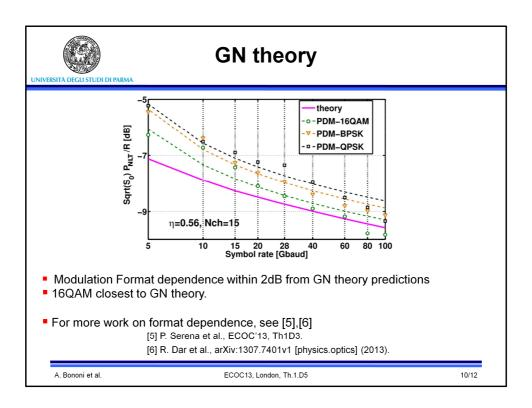
here is the plot of sqrt(S0) times NLT/R versus symbol rate.
