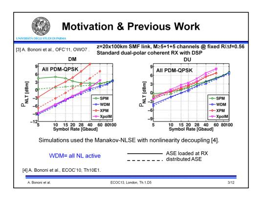
At OFC'11 we presented nonlinear threshold curves versus symbol rate R for both DM and DU cases.
