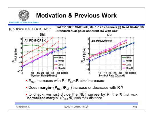
in both DM and DU cases the overall WDM NLT curves are increasing. Also the LT is increasing proportionally to R.
