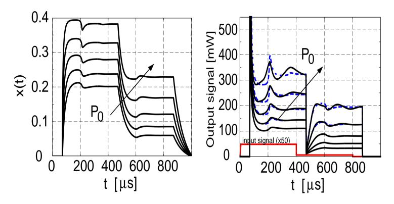
(Left) state variable, and (Right) output signal power, for increasing levels of pump power  $P_0 = 0.64, 0.70, 0.77, 0.86, 0.97$  W. Solid lines: exact solution (+DRB); Dahed lines: model.
