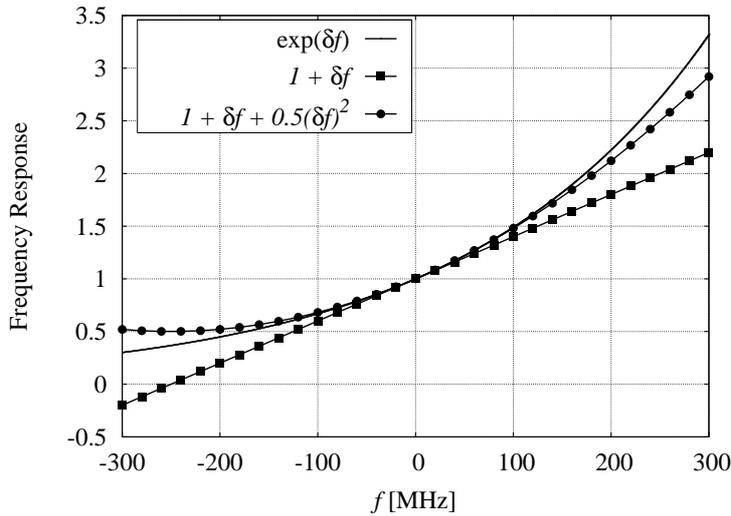
Fig. 1. Frequency responses of the exponential slope filter and of its first-order and second-order polynomial approximations, for  $\delta = 4$  ns.
