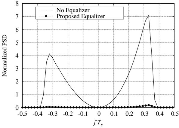
Fig. 7. Power spectral density of the difference among the signal as it should be after an ideal slope compensator and the signal as it really is in the absence/presence of the proposed equalizer.
