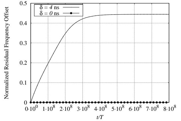
Fig. 8. Residual frequency offset, normalized with respect to the symbol rate, after an AFC loop implementing the ML algorithm, in the cases of strong slope ( $\delta = 4$  ns) and null slope ( $\delta = 0$  ns).
