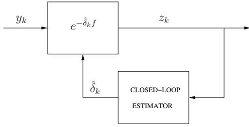
Fig. 3. Block diagram of the closed-loop equalizer.
