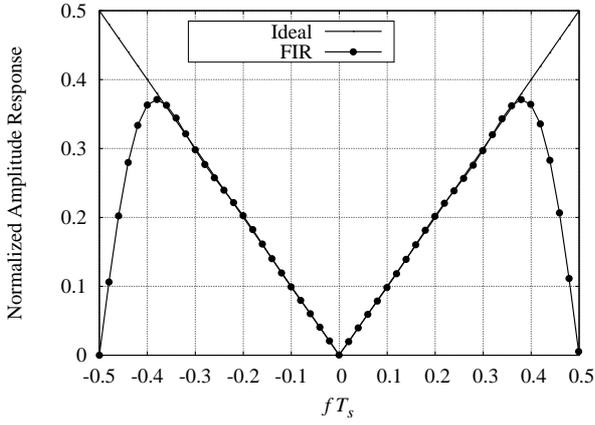
Fig. 5. Normalized amplitude responses of the ideal differentiator and of the considered FIR filter.
