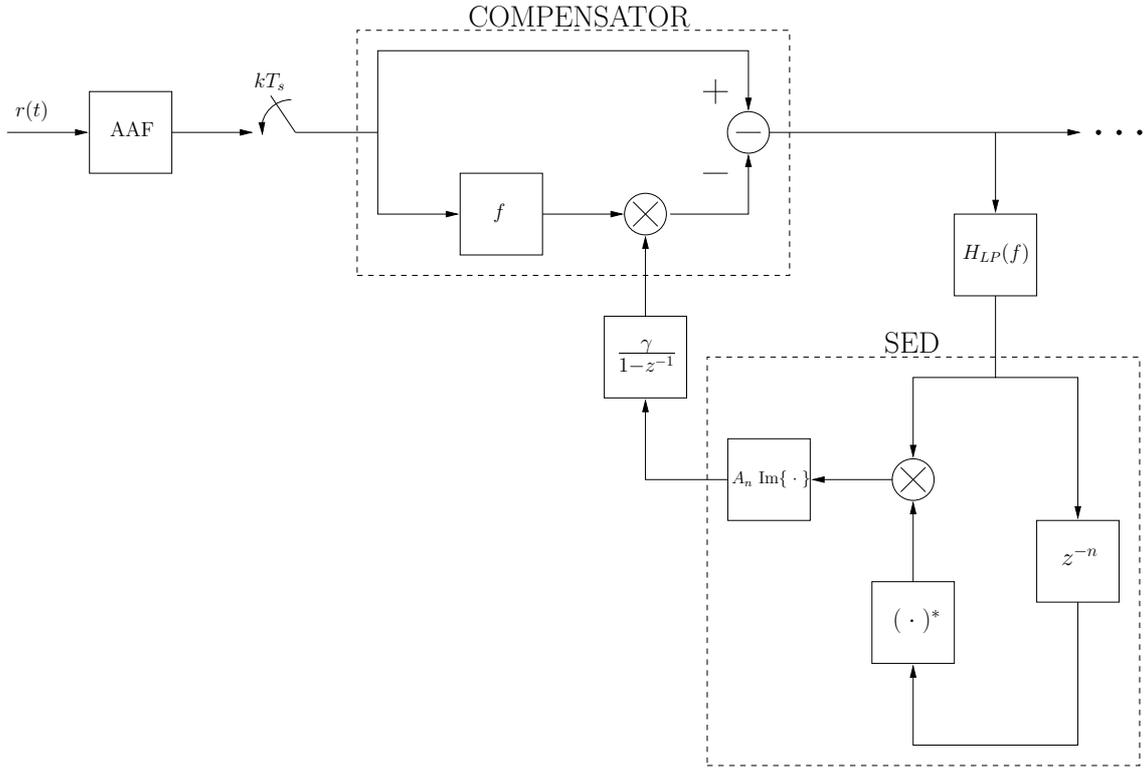
Fig. 9. Slope equalizer for systems where the received signal can be written as in (14).
