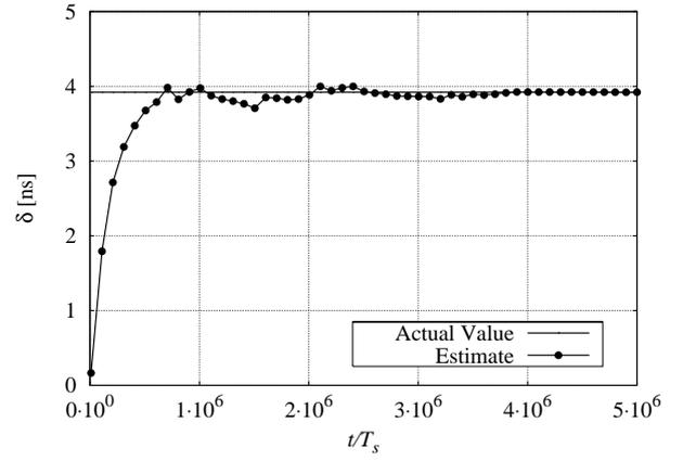
Fig. 6. Acquisition and tracking behavior of the proposed closed-loop equalizer.
