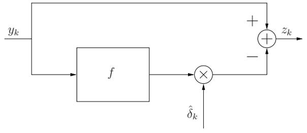
Fig. 4. Block diagram of the proposed low-complexity slope compensator.
