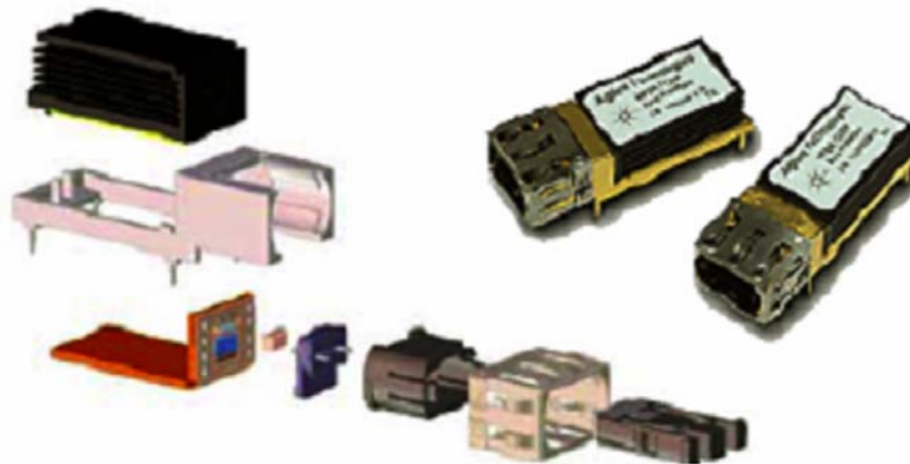
Figure 7. Typical server interconnect transceiver [9].
