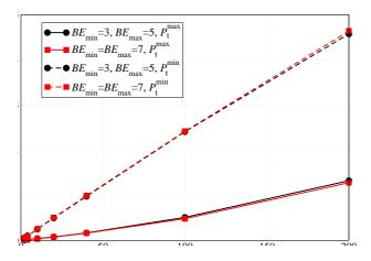
Figure 7. (a) Network transmission rate and (b) delay, as functions of the total offered traffic load (Ng), in the presence of (i) default backoff exponent, i.e.,  $BE_{\min} = 3$  and  $BE_{\max} = 5$ , and (ii) modified backoff exponent, i.e.,  $BE_{\min} = BE_{\max} = 7$ . Different values of transmit powers are considered. The allocated transmit power is the same at each node.
