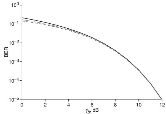
**Fig. 1** Upper and lower bounds for BER of DQPSK transmission with Gray coding over AWGN channel
