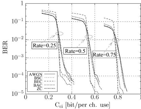
Fig. 3. BER versus constrained-input capacity for three LDPC codes, characterized by rates 1/4, 1/2, and 3/4, respectively. For each code, the performance for transmission over five memoryless channels is shown. The codeword length is 10 000 and the codes are optimized for transmission on the AWGN channel.
