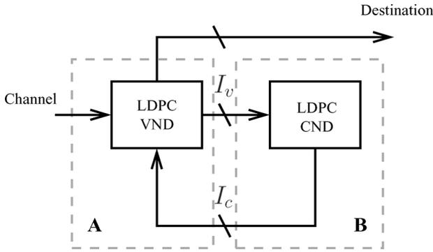
Fig. 1. Block diagram of an iterative receiver for LDPC-coded transmissions.
