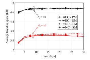
**Fig. 5.** Average free available disk space per StN, as a function of time, in a scenario with k = 50,  $T_{\rm M} = 30$  min,  $T_{\rm s} = 3$  min, and  $q = 2^{16}$ . Different coding and maintenance strategies are considered.
