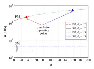
**Fig. 6.** Maintenance bandwidth, as a function of  $\phi$ , in a scenario with k = 50 with either PM with  $T_{\rm M} = 30$  min or SM with  $T_{\rm s} = 3$  min. Two values  $R_{\rm c}$  for the coding rate are considered: 1/2 or 1/5. Other parameters are obtained through simulations.
