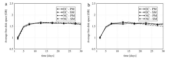
**Fig. 7.** Average free available disk space per StN, as a function of time, in a scenario with k = 50,  $R_c = 1/2$ ,  $T_M = 30 \text{ min}$ ,  $q = 2^{16}$ , and the non-uniform file size distribution. The performance is analyzed for both  $T_s = 3 \text{ min}$  (case (a)) and  $T_s = 36 \text{ s}$  (case (b)). Different coding and maintenance strategies are considered.
