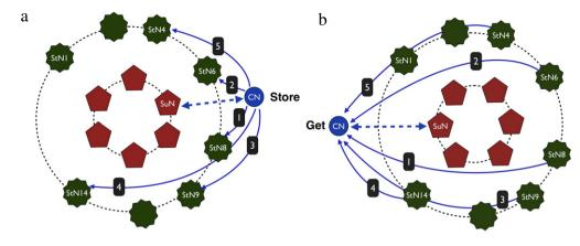
Fig. 1. The considered P2P overlay scheme with illustrative examples of (a) resource store and (b) resource retrieval process. In both cases, the resource consists of 5 fragments.
