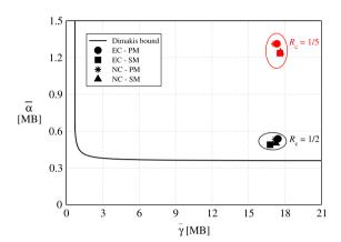
**Fig. 4.** Storage/repair tradeoff for resources of average size  $\overline{\mathcal{M}} = 18$  MB divided into 50 fragments coded with rate  $R_c = 1/2$  or  $R_c = 1/5$ . The operating points of different strategies are shown.
