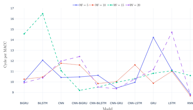
FIGURE 13. Comparison, in terms of number of cycles per MACC, between the considered ML and DL models for different values of the time lag \mathcal{W} .
