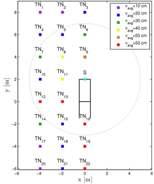
Fig. 3. The LGV (black rectangle) and its forks (black lines) are depicted together with the node,  $S$  (cyan star). The TN positions are also shown (colored squares). The colors are associated with the values of the average range error,  $v_{avg}$ . (For interpretation of the references to color in this figure legend, the reader is referred to the web version of this article.)
