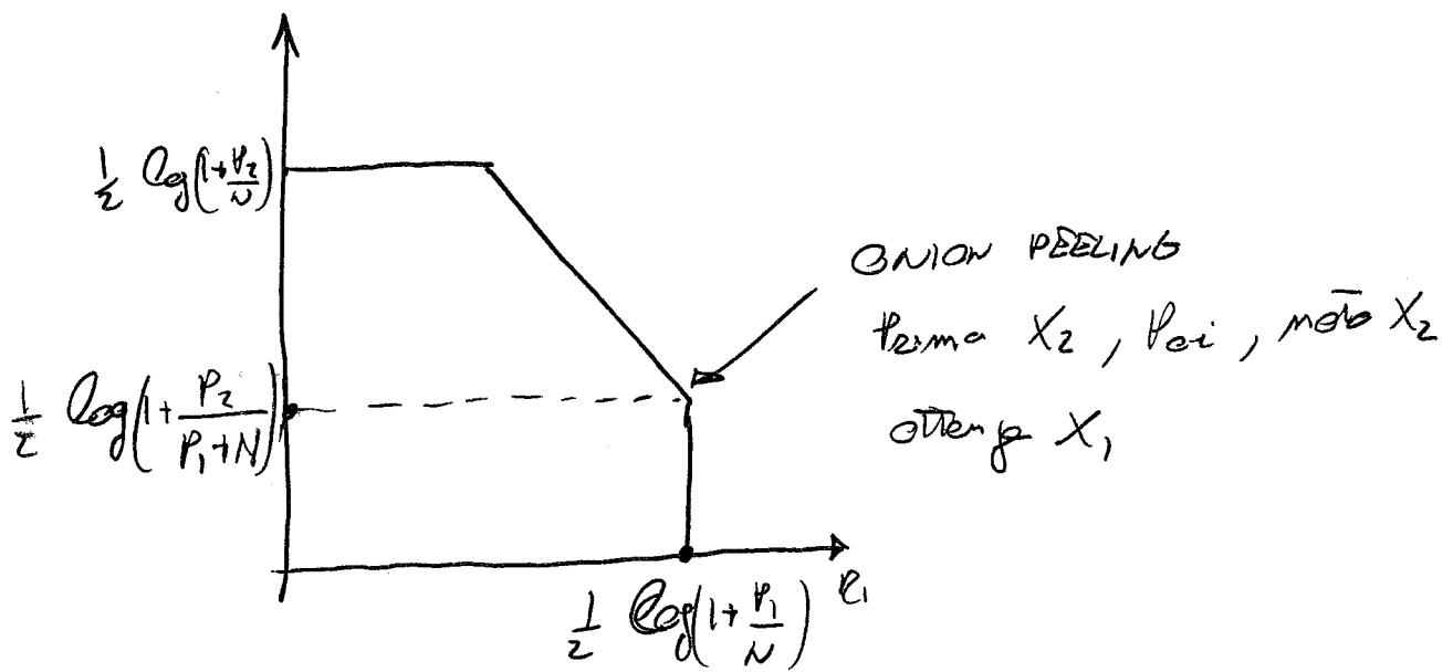
$$\left\{ \begin{array}{l} R_1 \leq \frac{1}{2} \log \left( 1 + \frac{P_1}{N} \right) \\ R_2 \leq \frac{1}{2} \log \left( 1 + \frac{P_2}{N} \right) \\ R_1 + R_2 \leq \frac{1}{2} \log \left( 1 + \frac{P_1 + P_2}{N} \right) \end{array} \right.$$
