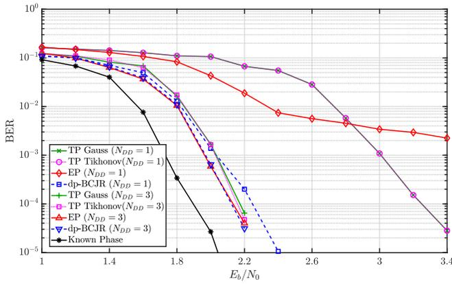
Fig. 2. Bit error rate curves for the tested algorithms, without ( $N_{DD} = 1$ ) or with ( $N_{DD} = 3$ ) detector-decoder iterations. The phase noise standard deviation is  $\sigma_{\Delta} = 6$  [deg] and  $(1/20)$  pilot symbols are distributed among the payload. In dp-BCJR, phase is discretized using  $N_{\theta} = 64$  levels.
