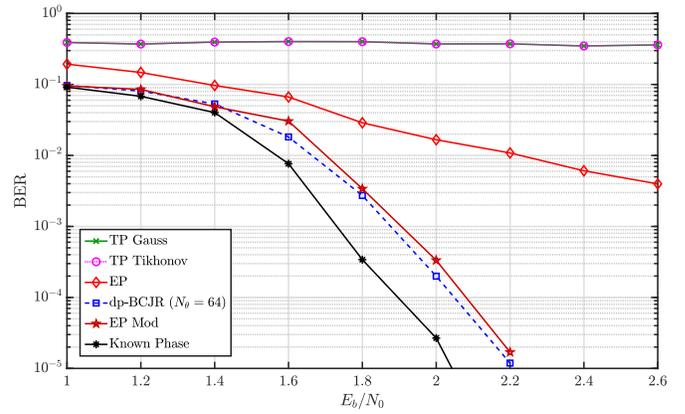
Fig. 3. Bit error rate curves for the tested algorithms, with separate detection and decoding ( $N_{DD} = 1$ ). The phase noise standard deviation is  $\sigma_{\Delta} = 3$  [deg] and  $(1/20)$  pilot symbols are concentrated in the preamble and postamble (half and half) of the transmitted packet. In dp-BCJR, phase is discretized using  $N_{\theta} = 64$  levels.
