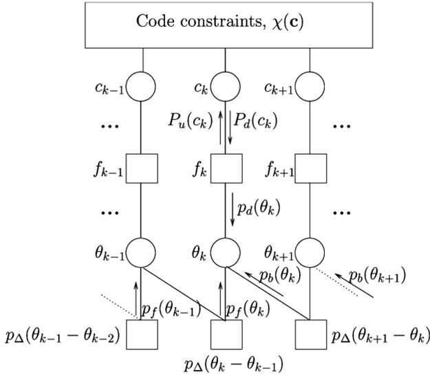
Fig. 1. Factor graph representing the joint probability distribution of phase noise samples and coded symbols.
