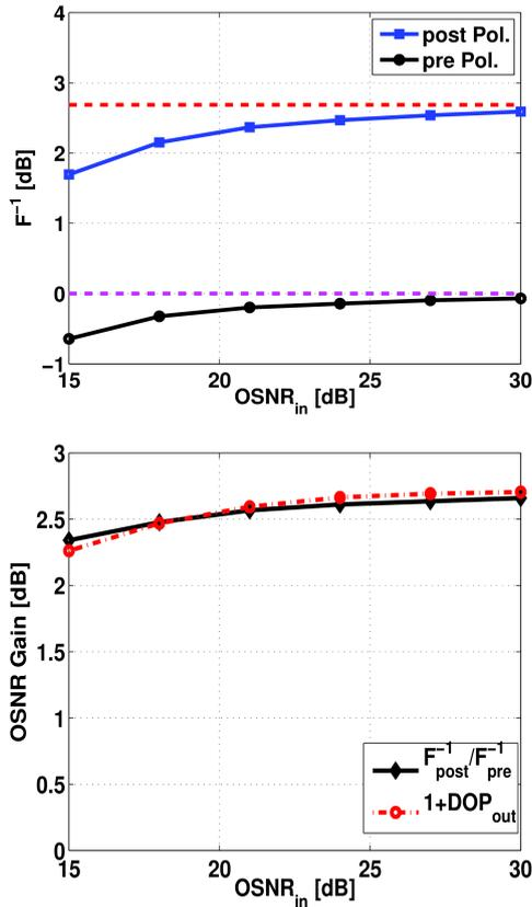
Fig. 2. (a) Inverse noise figure, measured before (*pre*) and after (*post*) the polarizer. (b) OSNR gain provided by LPA and its theoretical approximation.
