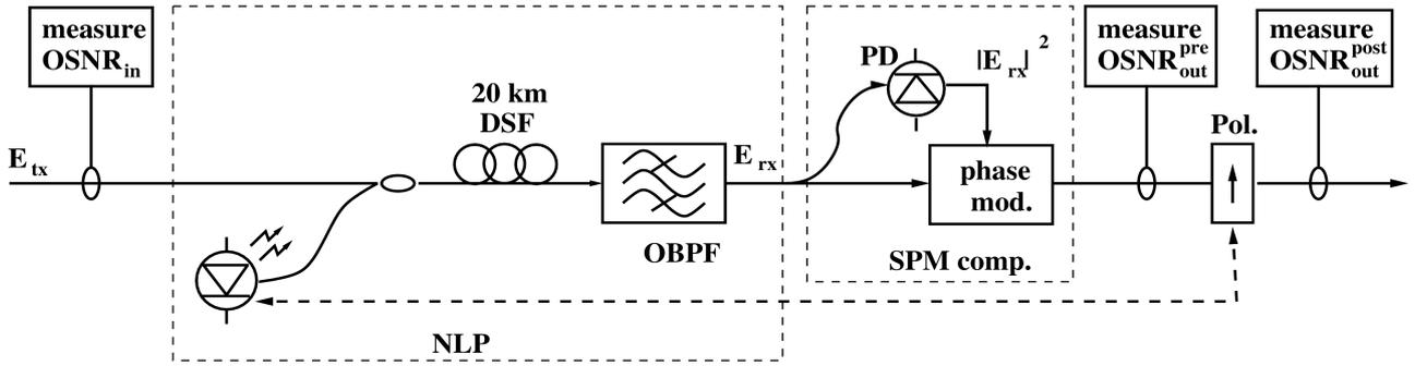
Fig. 1. Schematic setup of an all-optical noise cleaner. The nonlinear lossless polarizer (NLP) attracts the noisy signal towards the pump SOP; SPM compensation (SPM comp.) follows and, finally, an ideal polarizer (Pol.), aligned with the pump, removes the orthogonally polarized noise.
